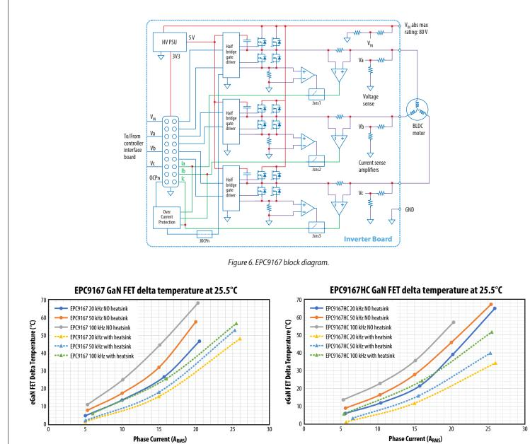
Figure 7. EPC9167 (a) and EPC9167HC (b) GaN FET temperature (\*) increase vs. the ambient temperature [25.5°C]. Measurements taken at various PWM frequencies. (\*) With heatsink, junction temperature has not measured directly. The indicated delta temperature with heat sink is the hottest point at the base of the heat sink.
