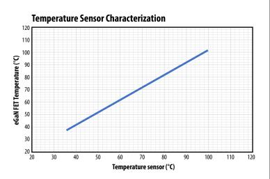
Figure 5. eGaN FET case temperature vs. temperature sensor placed on bottom of the PCB. Operation under natural convection without heatsink.
