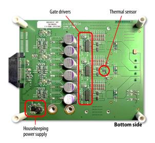
Figure 1. Photo overview of the EPC9167 EPC9167HC board highlighting the main sections.
