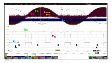
Figure 4. Phase and leg current sensing signals. Experimental waveforms during switching cycles and a zoomed view. The sampling point positions for the analog to digital signal are highlighted. Ia = 5 A/div,  $V_{DS, LS} = 50 V/div$ ,  $V_{RS} = V_{RSL} = 100 mV/div$ , t = 5 ms/div, zoomed view  $t = 10 \mu s/div$ .
